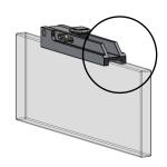
the beveled edge of the trigger always points toward the outer edge of the glass, i. e. in the direction of the door damper/end stop.
