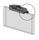
the beveled edge of the trigger always points toward the outer edge of the glass, i. e. in the direction of the cushioning/end stop.
